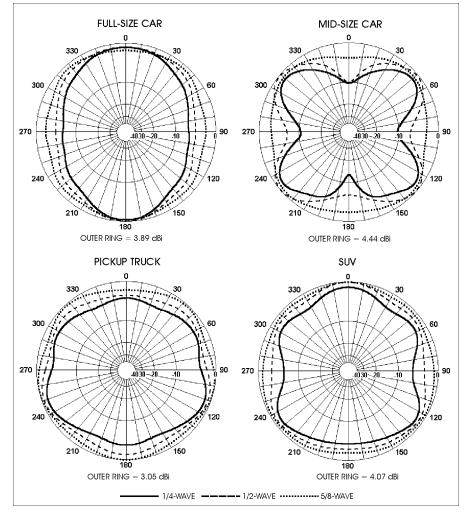
Figure 3 – Azimuth pattern variations (9° elevation) resulting with the different length antenna elements.
