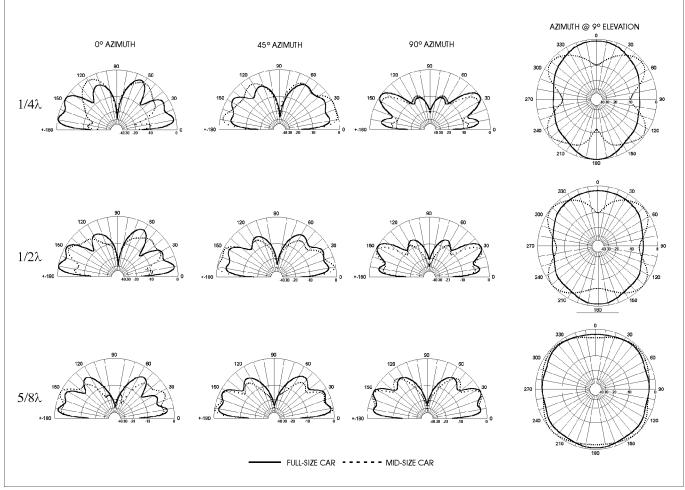
Figure 2 – Elevation and azimuth patterns showing the comparison between the full and mid-sized cars for the three most popular VHF mobile antennas
